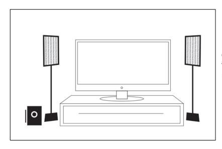
If your unit consists of the Amplifier/Woofer Combo Box with AC Power Supply, place it on the ground, centered below the two Emitters (see back view at top right). Do not block the sound port on front of the unit.
