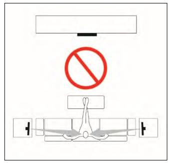
HSS sound is acutely directional. The Emitters must be set at the exact same angle from the Listener to achieve the optimal level of highly targeted sound. To ensure they are placed properly, first set them side-by-side. Direct the left Emitter toward the Listener's left ear, and the right Emitter toward the Listener's right ear. Adjust the Emitters so that they are at equal angles to the chair, as shown in the left diagram.
